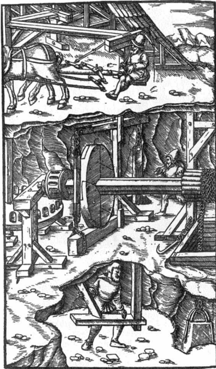
Horse-whim for raising large loads. The man below operates a brake consisting of a beam that can be lifted to bear on a drum fixed to the driving shaft. The load may be held stationary by catching the chain on a suspended hook. 1556. (Charles Singer, et al. A History of Technology, Vol. II, p. 18).
